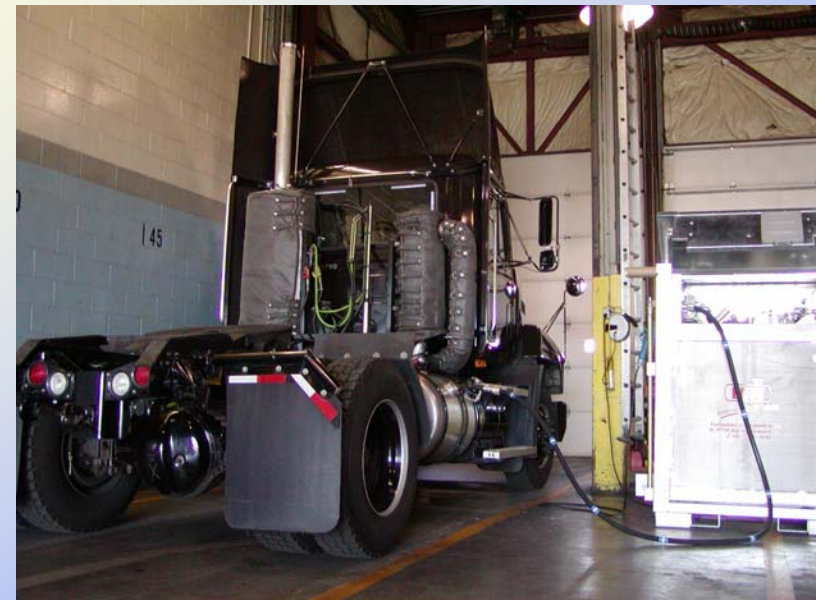
UPS SCR/DPF Combination Truck with Urea Filling Station
